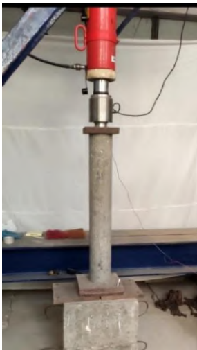
Fig. 4. Setup testing of the pile specimens.
