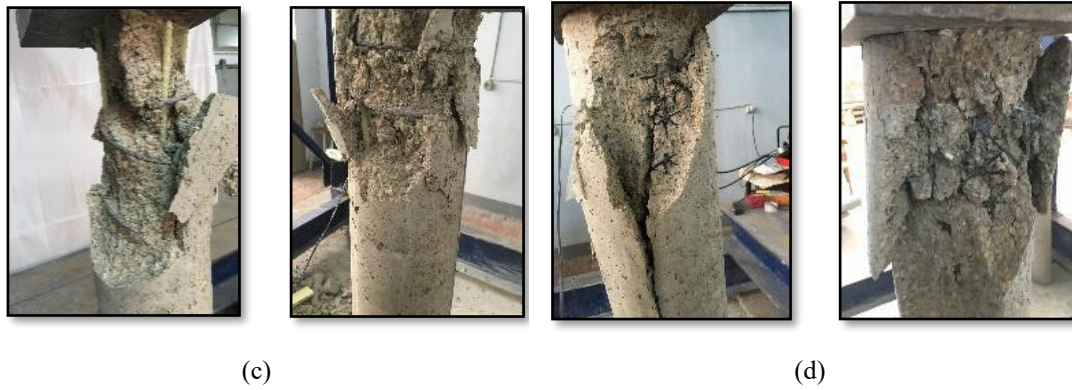
Fig. 5. Failure mode of tested specimens: (a) PS specimen, (b) PG specimens, (c) PGGB specimens, and (d) PGG specimens.
