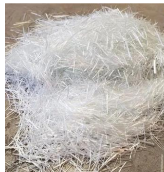
Fig. 1. Glass fibre bristles (GFB).
